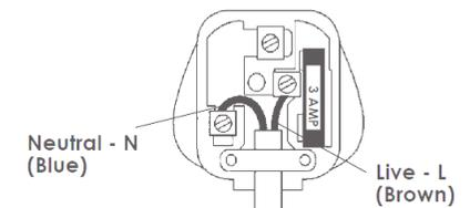
If a 13A (BS 1363) fused plug is used it must be fitted with a 3A fuse. If in doubt consult a qualified electrician.
